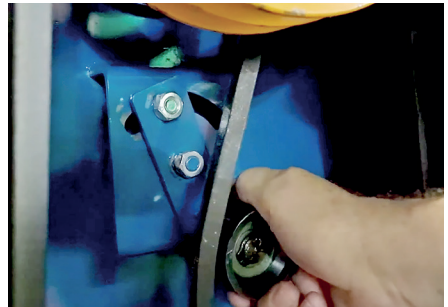
...and turn the bracket with the pulley against the belts, then retighten the nuts
