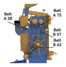
**C) Belt A 75** – Hulling Rollers Drive (fixed bearing):
