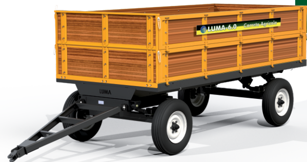
LUMA-6.0 Suspension by spring beam and floor and guards in Marine Plywood
